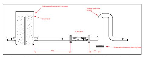
Length of straight sections of the pipeline
